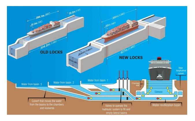
Diagram showing how water is used to fill or empty the lock chamber to raise or lower a ship. A lock canal was chosen because the other option, a sea-level canal, which would be a direct sea-level path between the oceans, would require too much digging.
